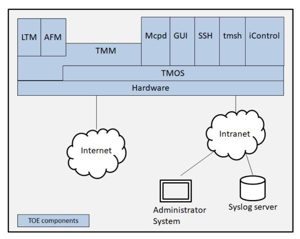
Figure 7: Architectural aspects of BIG-IP - F5 Device (except rSeries and VELOS) in Application Delivery Controller Deployments
