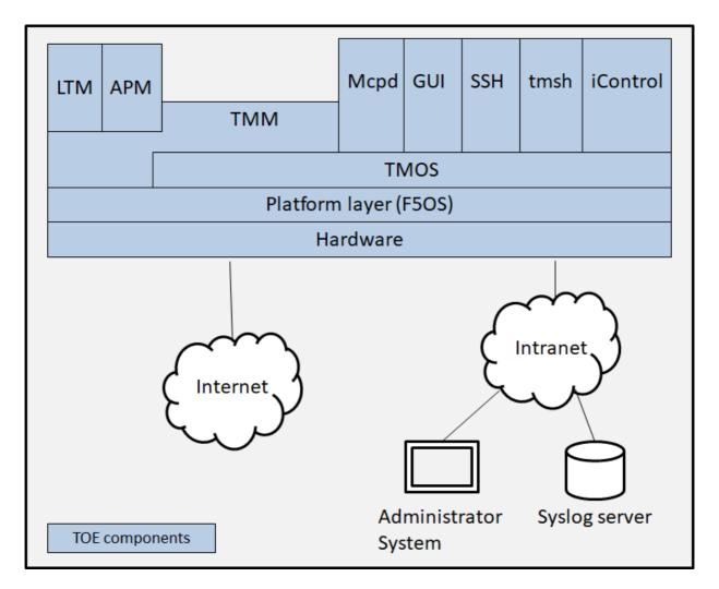
Figure 8: Architectural aspects of BIG-IP - F5 Device (except rSeries and VELOS) in Application Delivery Firewall Deployments
